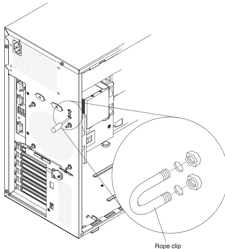
To install a rope clip, complete the following steps:
