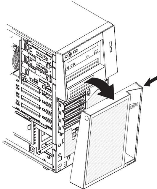
3. Lift the lower bezel to disengage the two bottom tabs from the chassis. Set the lower bezel aside.
