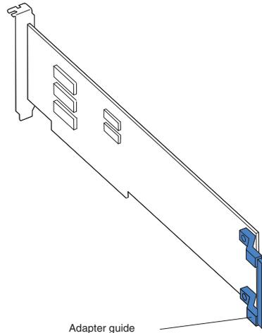
9. Carefully grasp the adapter by the top edge or upper corners, and align it with the expansion slot guides; then, press the adapter *firmly* into the expansion slot. Move the adapter directly from the static-protective package to the expansion slot.
