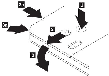
Using the tip of a ball point pen, push and break the lock pin tab **1**. To remove the disc, use a ball point pen to push down on the cartridge lid lock **2** and pull the cartridge lid out **3**. When the cartridge lid is open, the disc can be removed.
