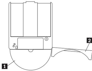
To return the disc to the cartridge, align the label side of the disc **1** with the DVD-RAM cartridge label side. Insert the disc and close the cartridge lid **2**. A clicking sound will occur when the lid closed.
