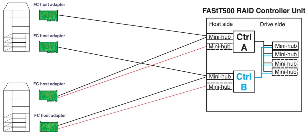
Figure 50. Type 2 configuration - With hubs
