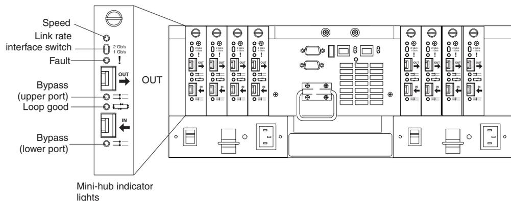
Figure 94. Type 1742 FASiT900 storage server mini-hub indicator lights
