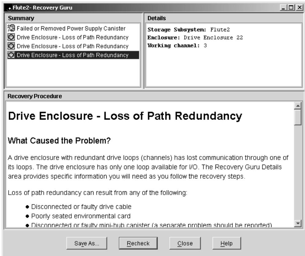
Figure 84. Recovery Guru - Loss of path redundancy
