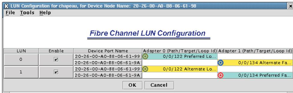
Figure 80. Preferred and alternate paths between adapters
