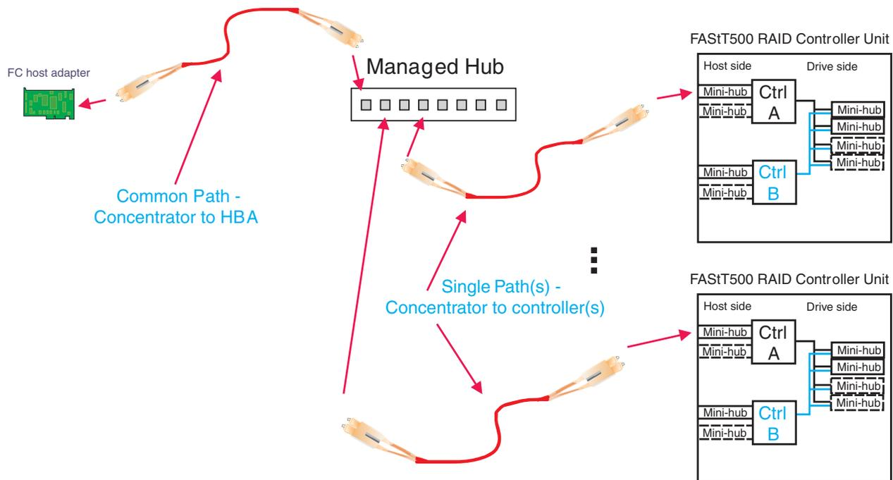
Figure 52. Type 2 configuration with multiple controller units
