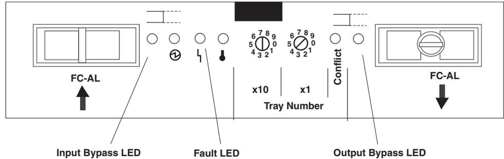
Figure 95. FAST EXP500 ESM indicator lights
