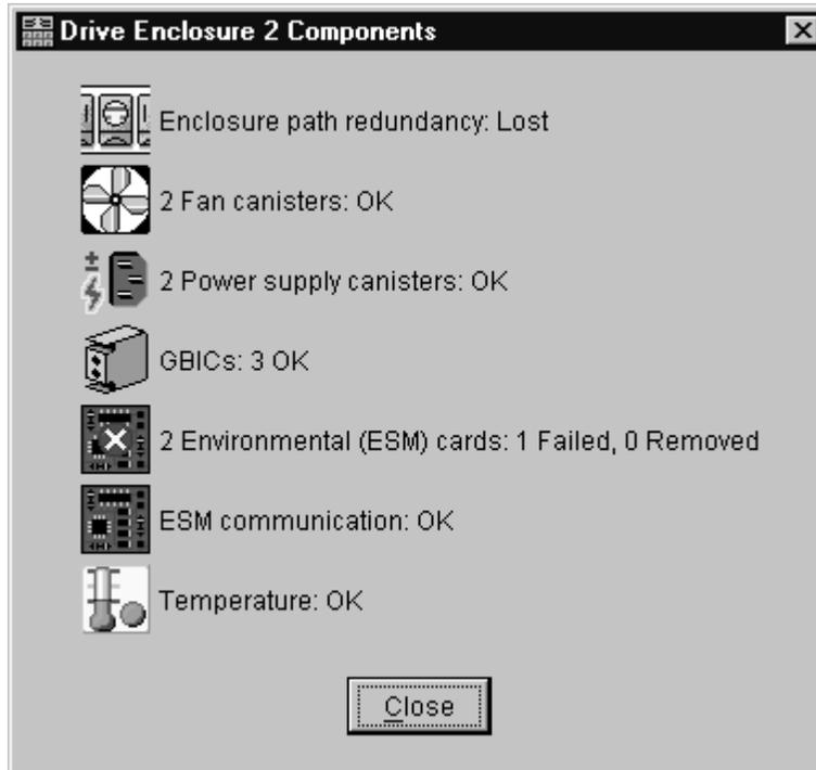
*Figure 82. Drive enclosure components - ESM failure*
