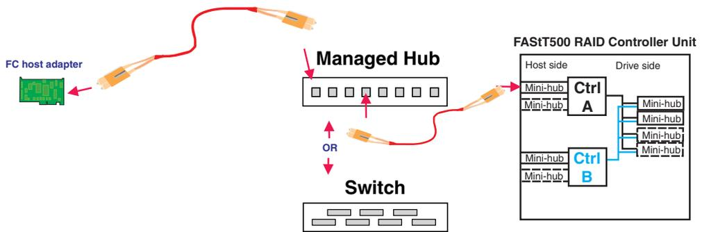
Figure 101. Typical connection path
