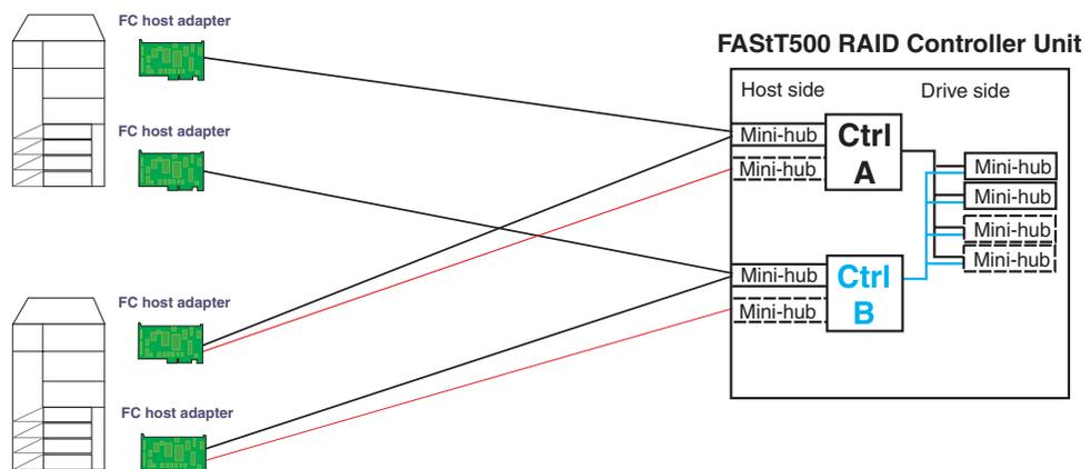
Figure 51. Type 2 configuration - Without hubs
