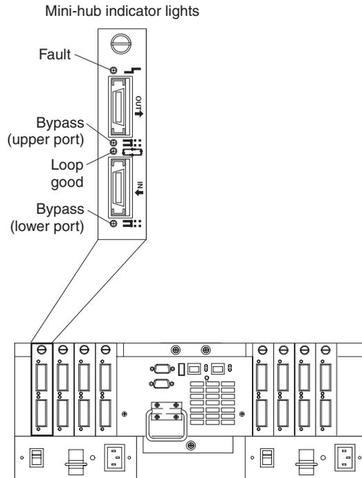
Figure 92. FAStT500 RAID controller mini-hub indicator lights
