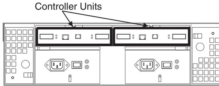
Figure 69. FAStT200 fibre channel controller unit locations
