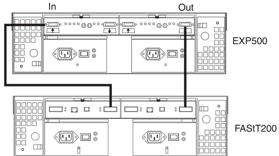
Figure 70. EXP500 and FAStT200 configuration
