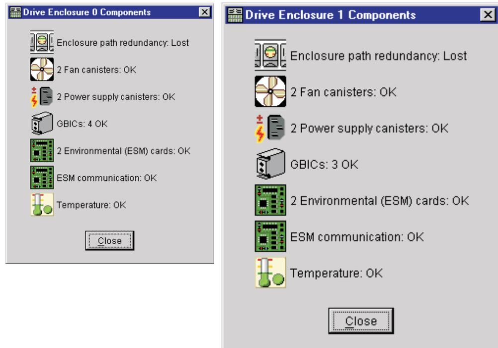
Figure 82 on page 194 shows that an ESM failed.
