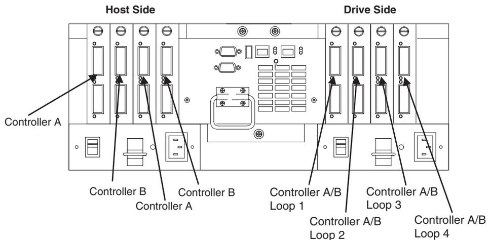
Figure 68. FASt500 controller connection locations
