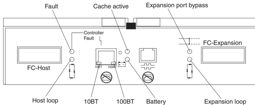
Figure 91. FAStT200 controller indicator lights
