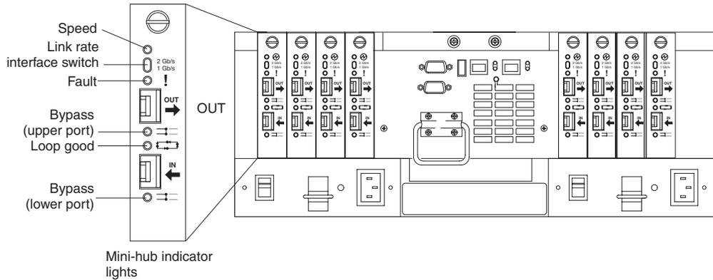
Figure 93. Type 1742 FAST700 storage server mini-hub indicator lights
