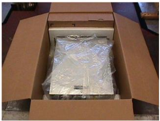
2.16 Break apart top cushion set (25P1115) and place on top front and rear edge of system.
