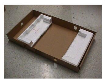
2.6 Leave about 5 inches of space for the shipgroup between the edge of the bottom tray and edge of front bottom cushion. The arrow (colored in red for clarity)on the front bottom cushion must always point toward the shipgroup.
