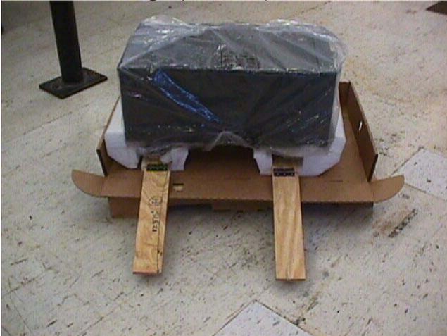
**2.10** Place tamper label (06P6550) on bag vertically (as shown) next to previously placed IBM logo tape to seal fold over edge of bag (**Do not place seal over tape**).
