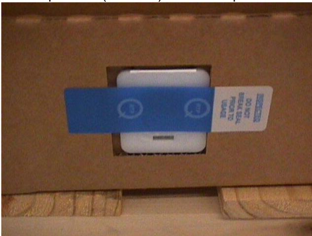
**2.15** Locate cushion ramps (01R3717) (2X) and slide down side of unit between wood ramps and carton. Make sure cushion is flush with the bottom of the tray and the wood ramps are pulled flush against the
