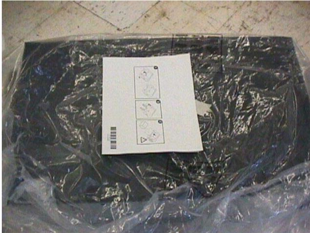
**2.18** Place top cushion (01R3716) on unit. Make sure the top front cushion and the top rear is cushion are in their respected places and that the tabs on the side of the cushions interlock with the cushion ramps. **Note: Top Front and Top Rear cushion come as a set that must be broke apart .**
