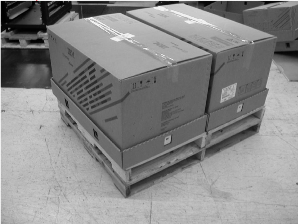
3.2 - Secure load to pallet utilizing "Best of Breed" palletization methods. See 92F6168 - "Best of Breed" Pallet Unitization or QMX document P-04146.
