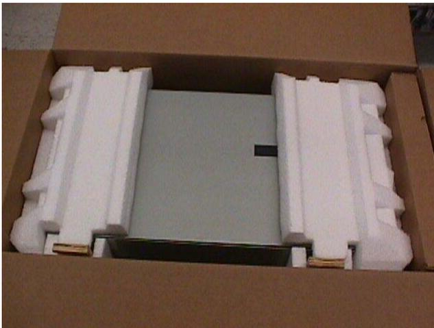
**NOTE: Do NOT place extra shipgroup items in voids around the system . Materials placed in these areas will result in damage to the system . IBM WW Packaging Engineering must be contacted if contents do not fit in the shipgroup area .**
