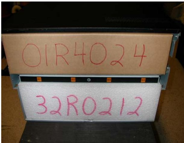
2.8 Place unit in bottom cushions. Make sure system is positioned all the way down and not sitting on the cushion ledge. Pull the bag up around the sides of the unit and fold neatly on top.
