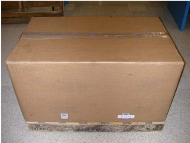
2.19 Place Intel label (if called out in DFC) on the top of the carton between label location marks.
