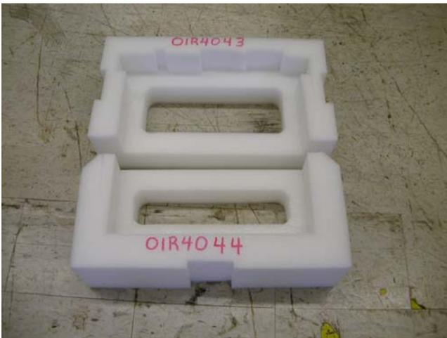
2.5 Place bottom front cushion (01R4043) in tray. Make sure bottom front cushion is placed in tray so the side cutouts on the cushion align with front, side clip holes in tray and leave approximately 4.5 inches of space between the front cushion and front edge of bottom tray. Place bottom rear cushion (01R4044) all the way to the back of the tray.
