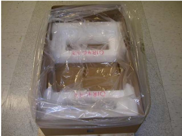
2.7 Place load spreader (01R4024) inside the top void in the rear of the unit. Place load spreader (32R0212) inside the bottom void in the rear of the unit.
