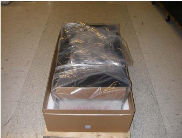
2.9 Use Tamper Label (06P6550) to seal edges of bag closed. Make sure bag is pulled tight.
