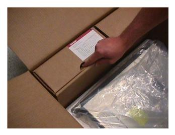
2.15 Break apart top cushion set (06P6552) and place on top front and rear edge of system.
