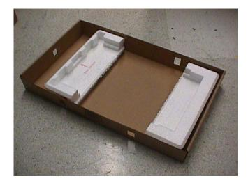
2.6 Leave about 5 inches of space for the shipgroup between the edge of the bottom tray and edge of front bottom cushion. The arrow (colored in red for clarity)
