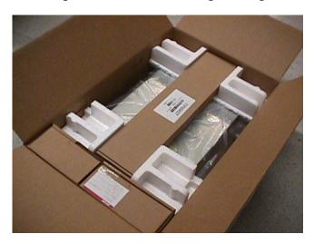
2.19 Close the top of the carton and seal using printed tape (74F5699 - Automatic taper, 74F5698 - for hand held dispensers).
