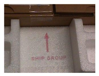
2.17 Place rack hardware kit on top of cushions inside center cavity.
