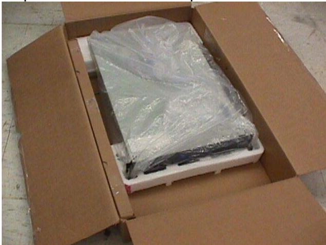
**Note:** This is how the corrugate Shipgroup Tube (01R3709) folds up to fit in front of the unit. Make sure that the edge with the cut-out tabs is place up in the pack.
