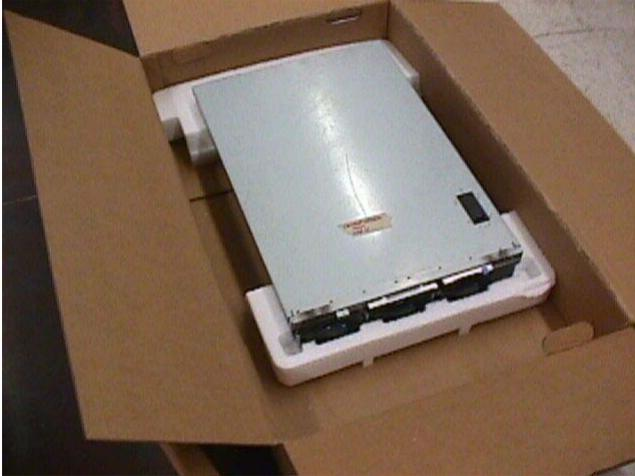
**2.7** - Insert the Rail Kit Carton (01R3711) on the left side of the unit in between the cushions and corrugate carton. As shown in the picture.
