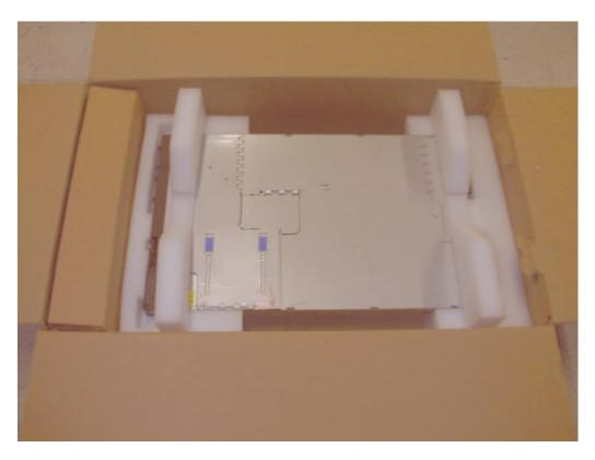
1.10 - Place rail kit on top of system as shown below.Note: Actual rail kit length may vary . Use hole in shipgroup for longer rail kits, if necessary .
