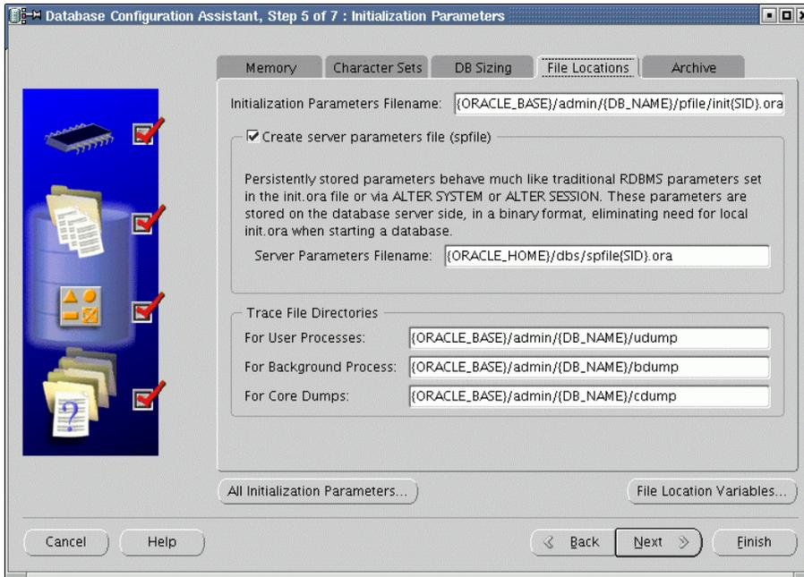
Figure 31. Database initialization parameters - file locations
