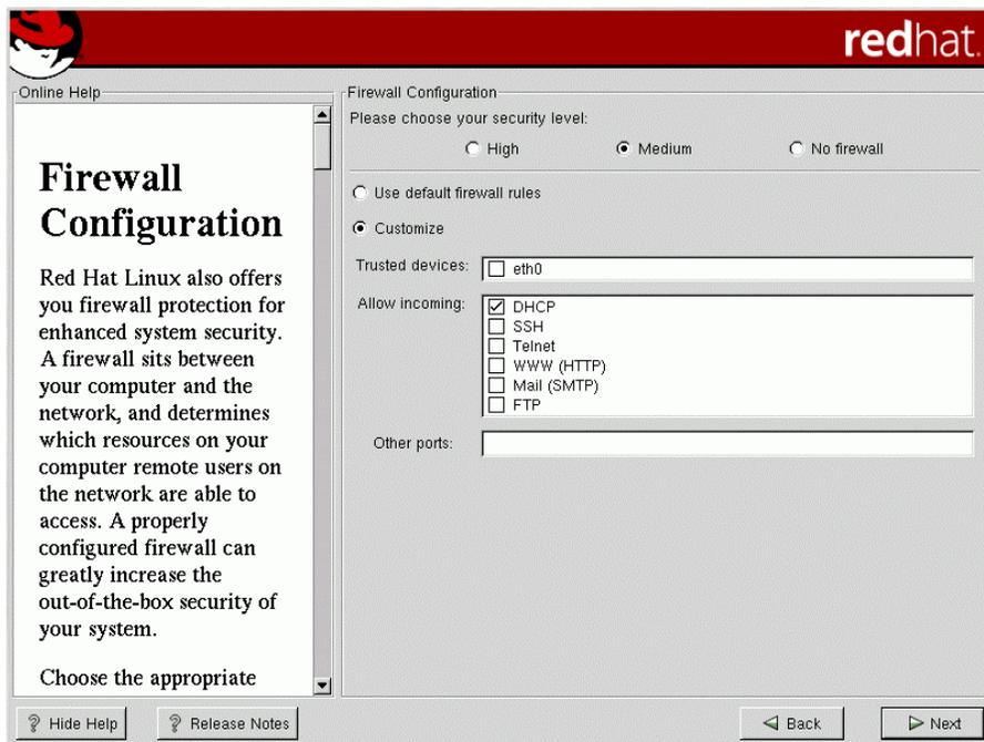
Figure 5. RHAS Firewall Configuration
