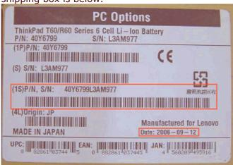
2. Option boxes may also be opened to view the part number and barcode. If the label on the battery displays one of the Assembly or FRU part numbers listed in the table above, you must use the 22-character 11S bar code number to determine whether or not the battery has been recalled. Lenovo has developed a Web tool to analyze whether or not a given battery has been recalled. Go to: www.lenovo.com/batteryprogram and follow the directions on the page.
