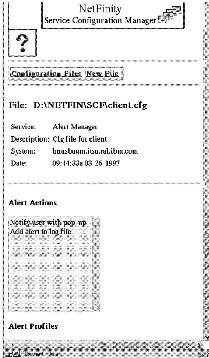
Figure 98. Service Configuration Manager - Edit Configuration File (Top)
