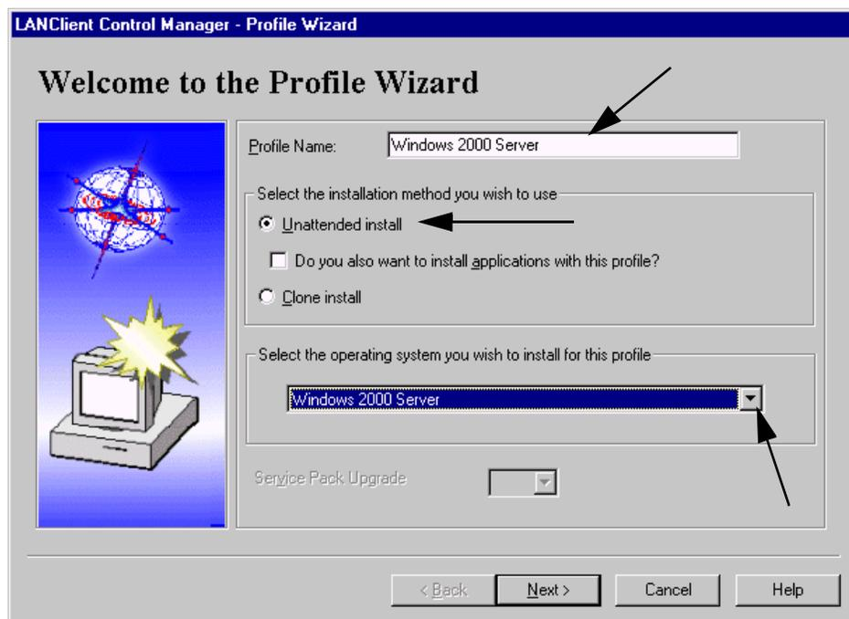
Figure 299. Setting installation details for the Windows 2000 Server profile
