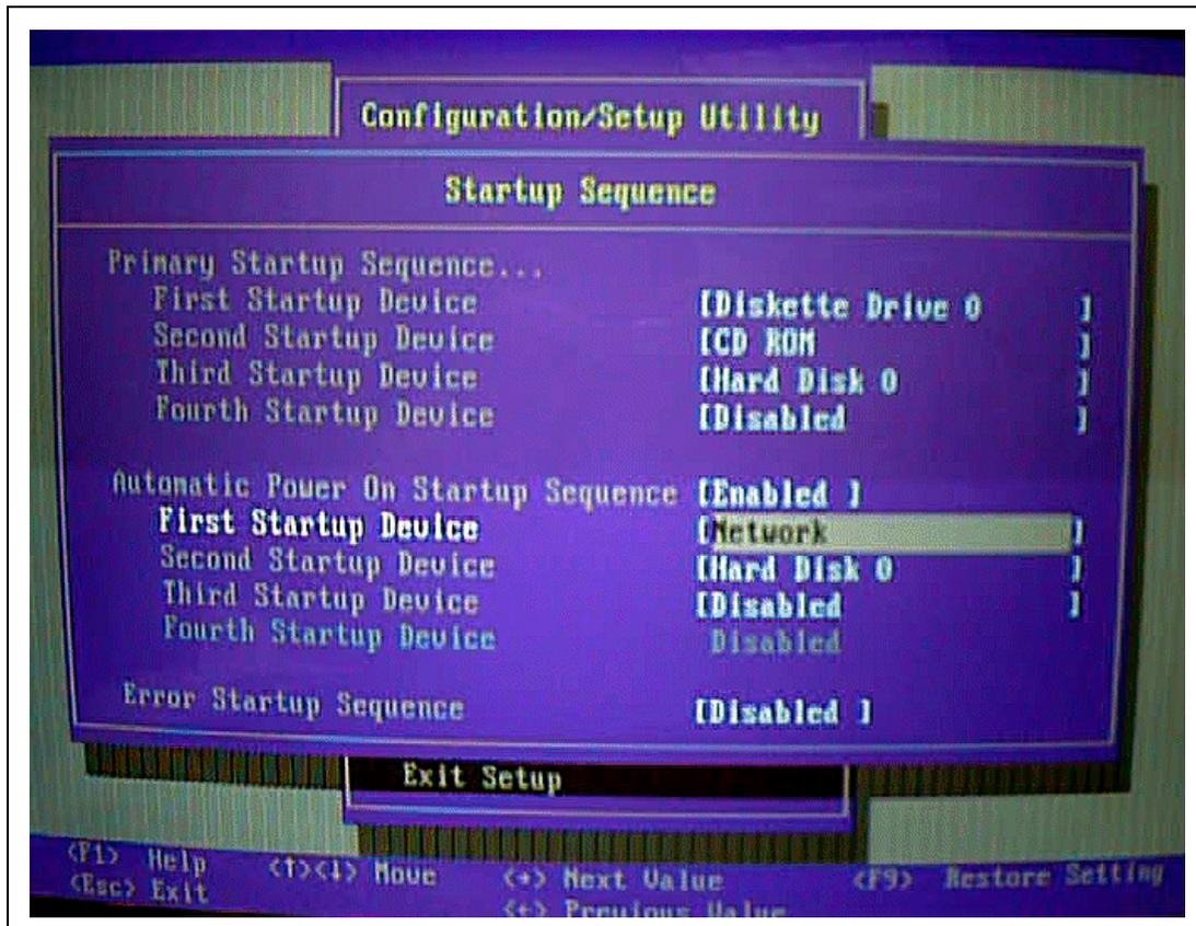
Figure 169. Startup sequence of Netfinity 3000 machine
