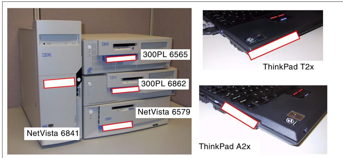
Figure 8. Asset ID antenna locations on various IBM systems
