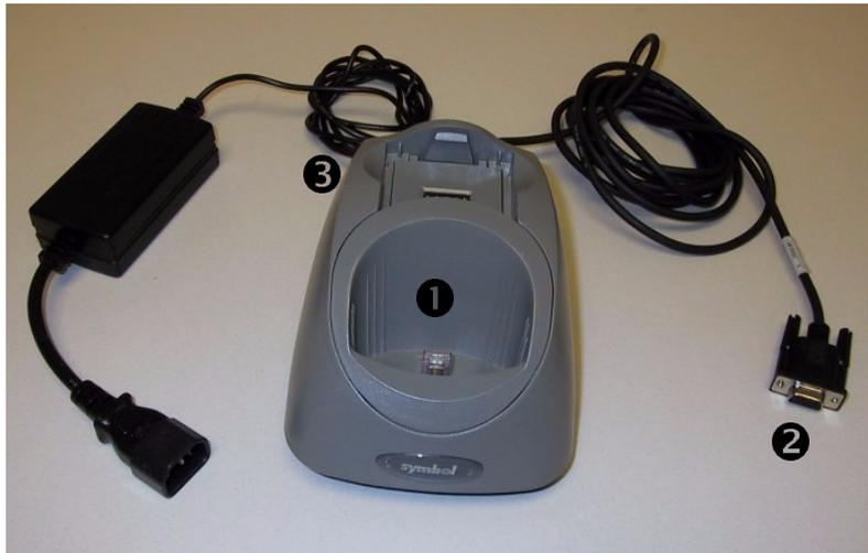
Figure 4. Recharger and host connection cradle
