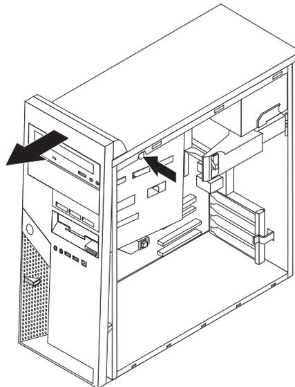
3. Remove the knockout from drive bay 3 by using a flat-blade screwdriver to pry it loose.
