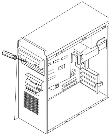
4. Remove the plastic panel in the bezel for bay 2 by squeezing the plastic tabs that secure the panel on the inside of the bezel.
