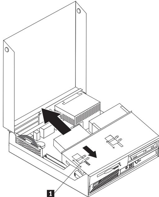
3. Slide the drive towards the rear of the computer far enough to gain access to the flat cable connector on the drive and disconnect the flat cable from the drive.
