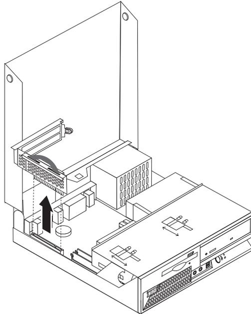
3. Release the slot cover latch and remove the slot cover for the appropriate expansion slot.
