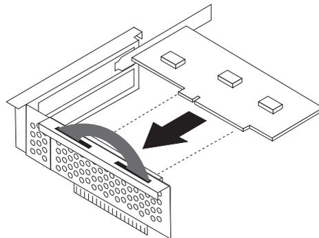
**Note:** The top slot is for the PCI adaptor and the bottom slot is for the PCI express adaptor.
