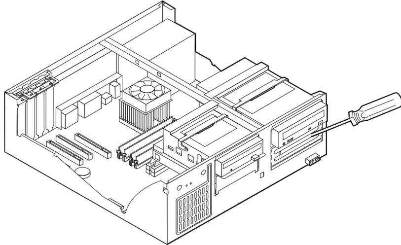
5. Pivot the drive-bay latch handle toward the front of the computer and then pivot the drive-bay cage upward, as shown, until it is latched in the upright position.
