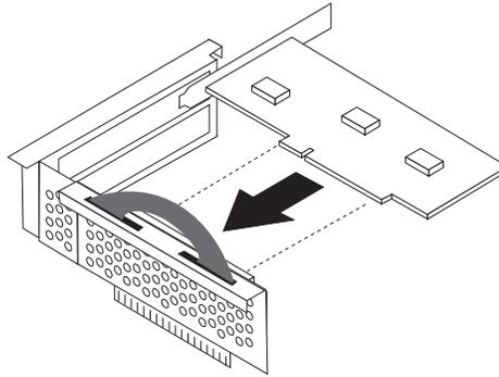
6. Position the adapter latch to retain the adapters.
