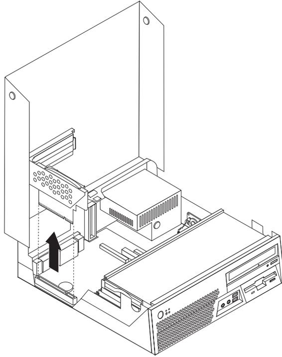
3. Release the adapter latch and remove the connector cover for the appropriate expansion connector.
