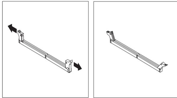
5. Position the memory module over the memory connector. Make sure that the notch **1** on the memory module aligns correctly with the connector key **2** on the system board. Push the memory module straight down into the connector until the retaining clips close.
