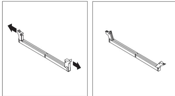
6. Position the memory module over the memory connector. Make sure that the notch **1** on the memory module aligns correctly with the connector key **2** on the system board. Push the memory module straight down into the connector until the retaining clips close.
