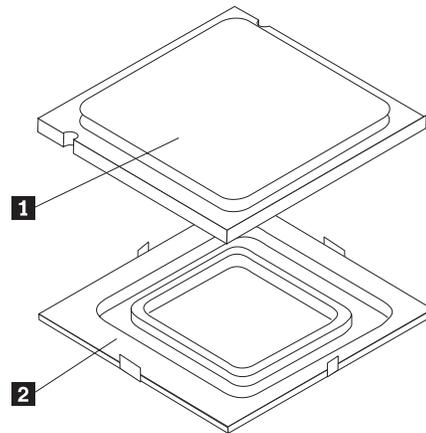
10. Position the microprocessor so that the notches on the microprocessor are aligned with the tabs in the microprocessor socket.
