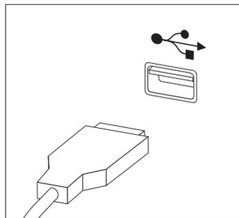
4. Disconnect the failing mouse cable from the computer.
