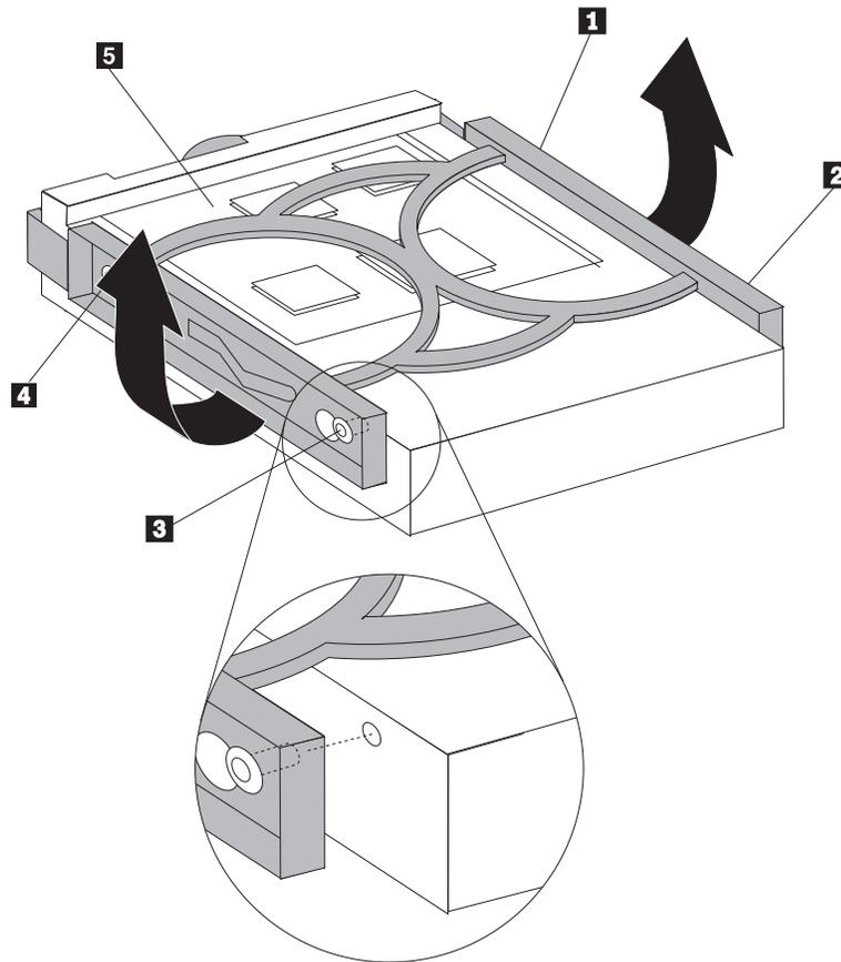
7. Insert the new hard disk drive into the hard drive bay until it snaps into position.
