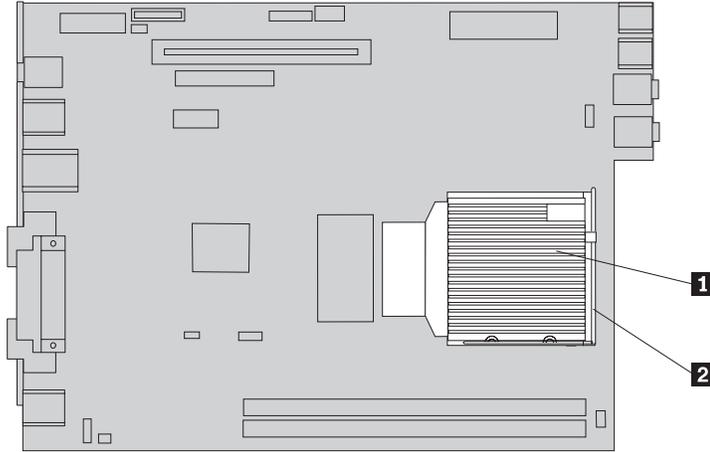
10. Use the handle at the rear of the system board to pull the system board and tray out the rear of the chassis.
