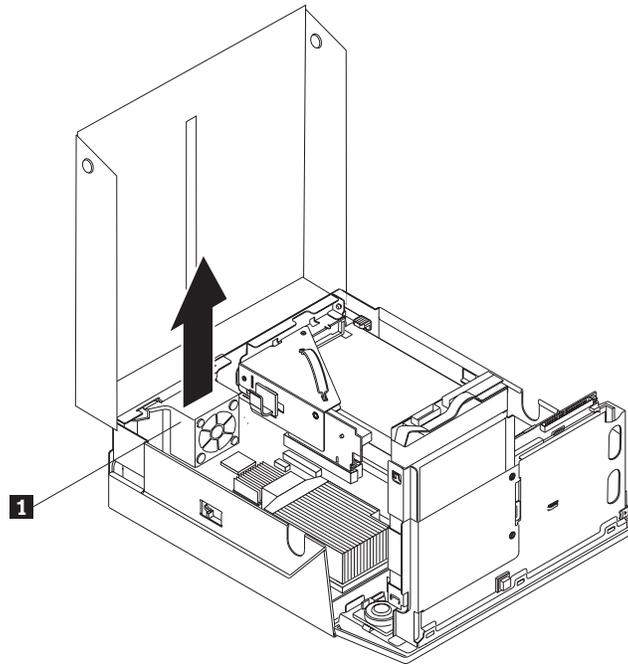
5. Remove the failing hard disk drive from the blue bracket by flexing the bracket enough to slide the drive out.
