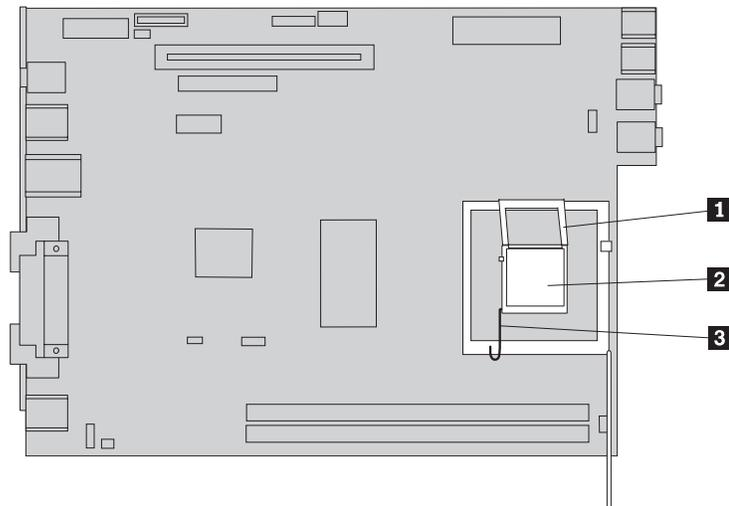
13. Place the new heat sink **1** into position and lower the lever **2** to secure the heat sink.
