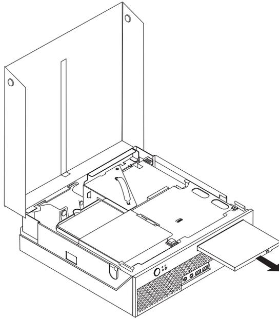
5. Slide the new optical drive into the bay until it locks into position.
