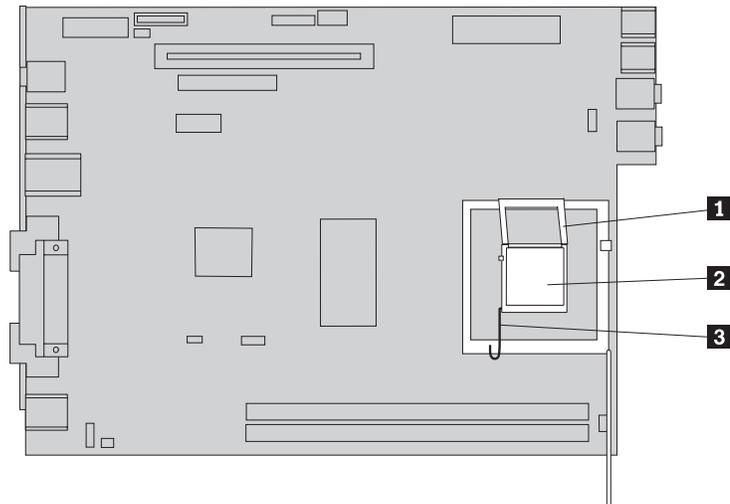
7. Remove the microprocessor from the system board socket by lifting it out of the socket.
