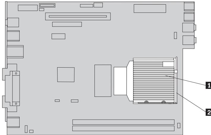
14. Reconnect the microprocessor fan cable to the system board.
