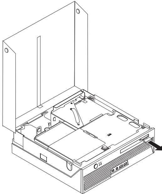
4. Slide the optical drive out of the front of the computer.
