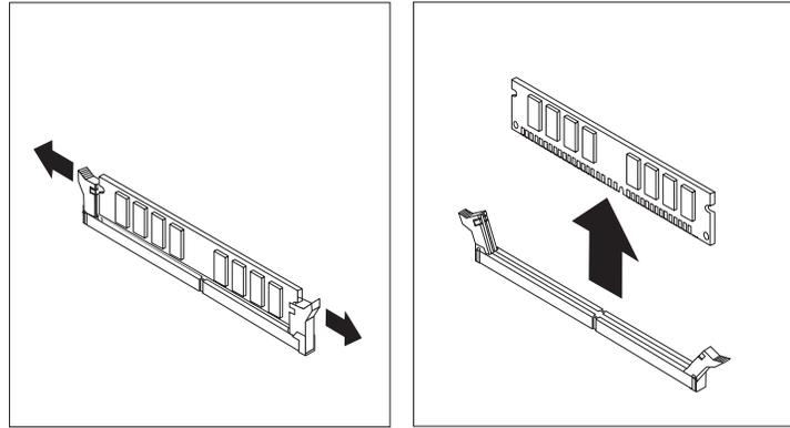
5. Position the replacement memory module over the memory connector. Make sure that the notch **1** on the memory module aligns correctly with the connector key **2** on the system board. Push the memory module straight down into the memory connector until the retaining clips close.
