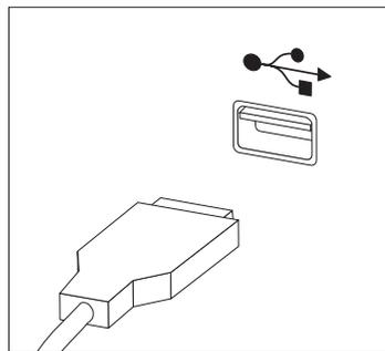
4. Disconnect the failing keyboard cable from the computer.
