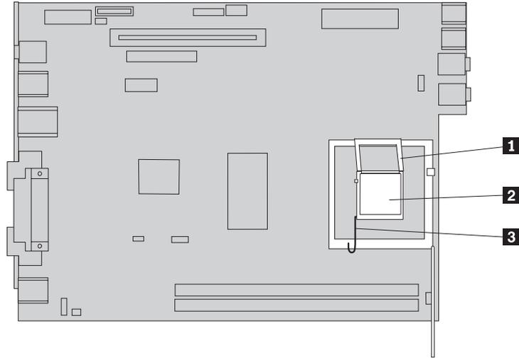
13. Remove the microprocessor from the system board socket by lifting it out of the socket.
