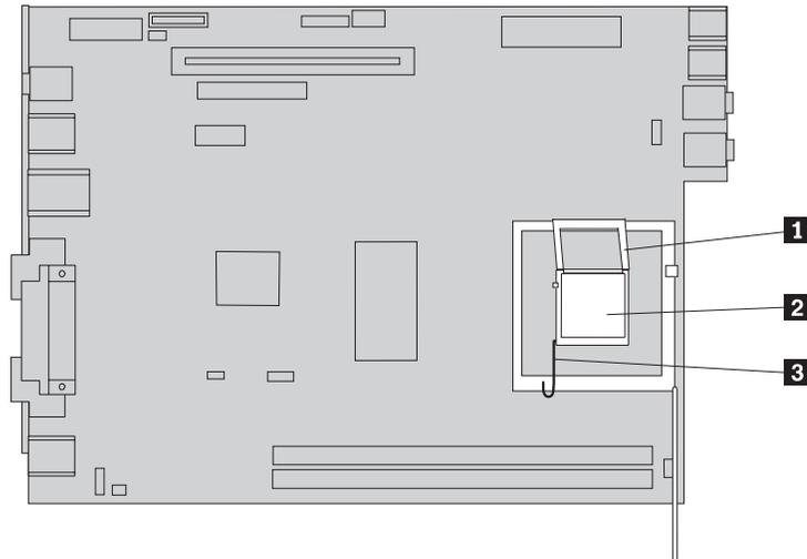
**Note:** There will be a black plastic cover on the microprocessor retainer to protect the socket on the new system board. When you lock the microprocessor in position, remove the black plastic cover. Place the black plastic cover on the microprocessor retainer of the failing system board.
