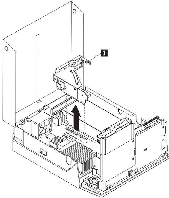
6. Pivot the adapter latch upward and remove the failing adapter.
