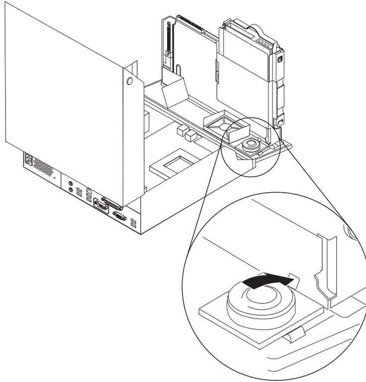
6. Position the bottom of the new speaker into the metal tabs then pivot the top of the speaker downward until it snaps into position.
