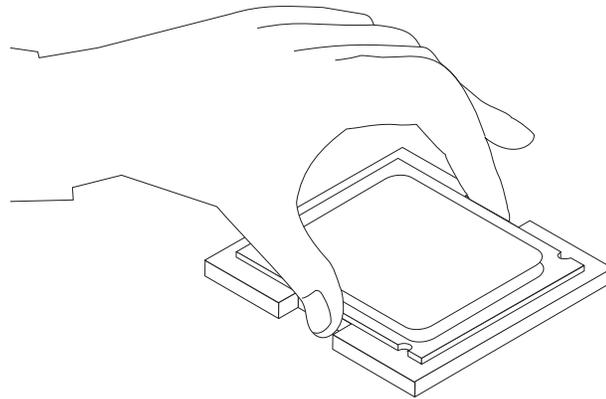
12. Lower the microprocessor retainer **1** and then lower the lever **3** to secure the retainer. Make sure the lever is securely locked into position.
