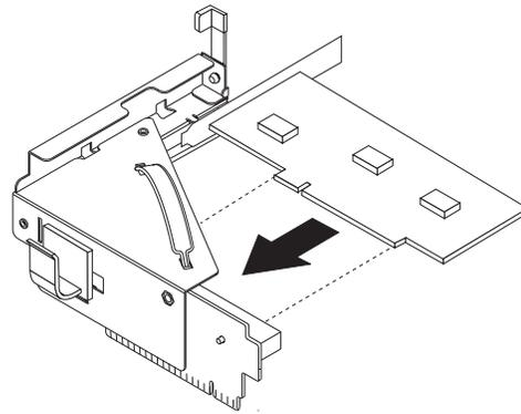
9. Pivot the adapter latch down to retain the adapter.
