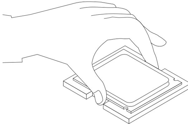
17. Lower the microprocessor retainer **1** and then lower the lever **3** to secure the retainer. Make sure the lever is securely locked into position.
