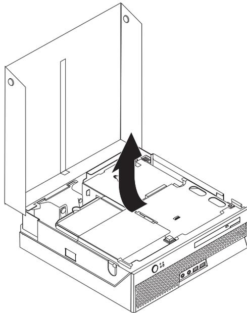
3. Remove the PCI riser. See “Replacing a PCI adapter” on page 27.
