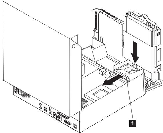
7. Install the new system fan and connect the system fan cable to the system board.
