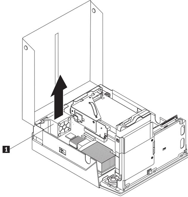
6. Install the new rear fan bracket assembly and connect the rear fan cable to the system board.
