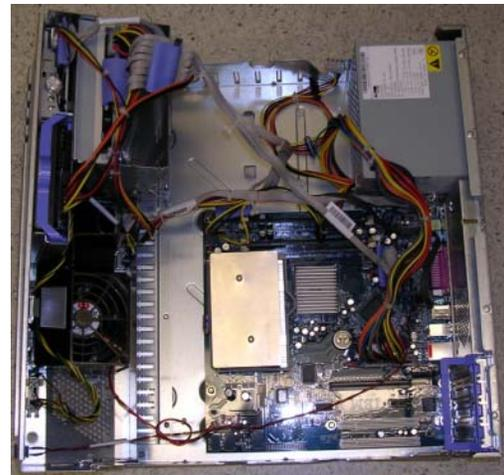
**Step 3:** An improperly installed board will have a deformation in the area of the board as depicted below. The system board will be slightly bent away from the wall of the chassis near the processor. For positive identification, continue to step 4.
