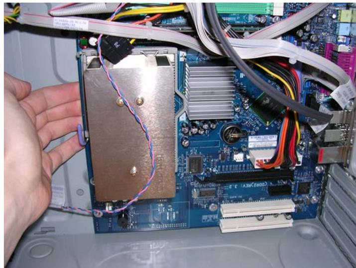
**Step 5 (board replacement, if necessary):** *If a system board is to be replaced, ensure that the system board is properly fit into the chassis. The system board needs to be slid into position such that the CPU retention module slides into the retention clips of the chassis. After sliding the system board (right to left in below picture), lift up on the board to ensure that the board is properly installed. A properly installed board will be securely locked to the chassis wall.*
