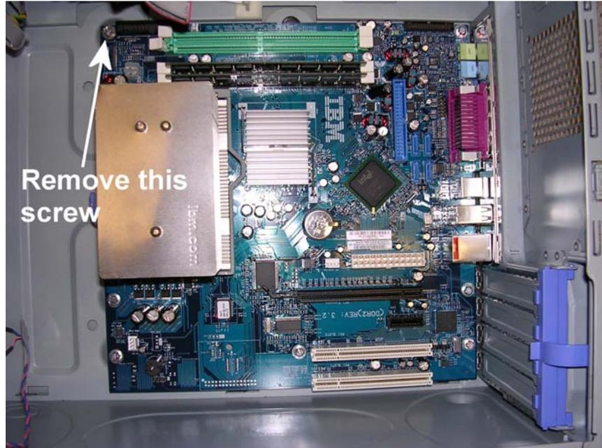
*Apply gentle upward pressure under the motherboard near the CPU and heatsink as shown below. Watch the corner of the system board where the screw was removed. If the corner of the board is easily lifted off the screw post, the board was improperly installed and should be replaced. A properly installed board will be locked in place, and not lift off the screw post.*
