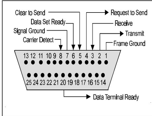
RS-232-C Host/Printer Port 1 Pin Assignments
