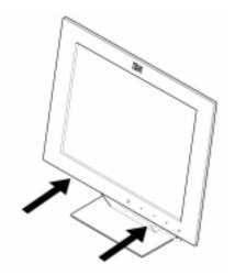
2. Before using your monitor for the first time, remove the clear protective film from the front of the screen.
