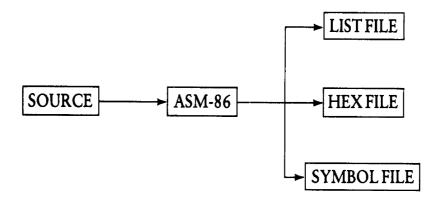
Figure 1-1. ASM-86 Source and Object Files
