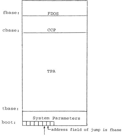
entry: the principal entry point to FDOS is at location 0005 which contains a JMP to fbase. The address field at location 0006 can be used to determine the size of available memory, assuming the CCP is being overlayed.
