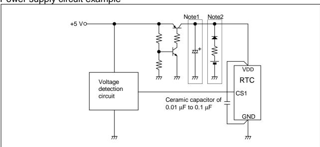
Note 1:This capacitor must be of a high capacity because a transient reverse current flows from the collector to the emitter of the transistor when the power is turned off.
