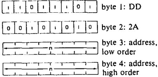
*Descriptions:* The contents of the memory location addressed by the memory locations immediately following the opcode are loaded into the low order of the IX register. The contents of the memory location immediately following the one loaded into the low order are loaded into the high order of the IX register. The low order of the nn address immediately follows the opcode.
