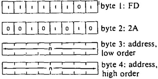
*Description:* The contents of the memory location addressed by the memory locations immediately following the opcode are loaded into the low order of the IY register. The contents of the memory location immediately following the one loaded into the low order are loaded into the high order of the IY register. The low order of the nn address immediately follows the opcode.
