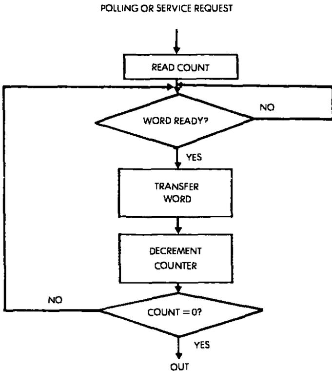
**Fig. 6.5: Parallel Word Transfer: Flowchart**
