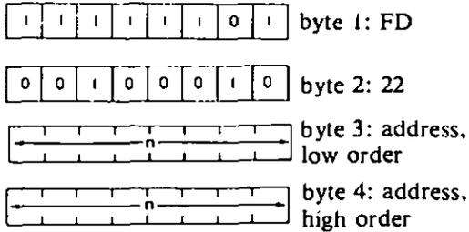
*Description:* The contents of the low order of the IY register are loaded into the memory location addressed by the contents of the memory locations immediately following the opcode. The contents of the high order of the IY register are loaded into the memory location immediately following the one loaded from the low order. The low order of the nn address occurs immediately after the opcode.
