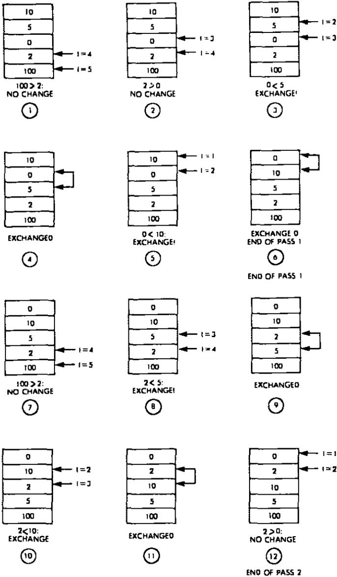
Fig. 8.5: Bubble-Sort Example: Phases 1 to 12
