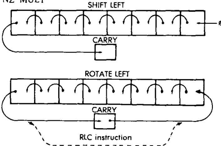
Fig. 3.17: Shift and Rotate
