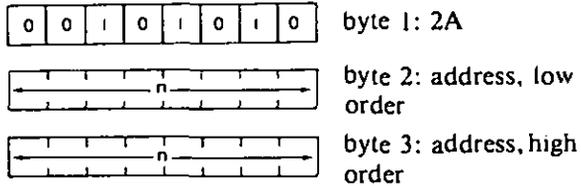
*Description:* The contents of the memory location addressed by the memory locations immediately after the opcode are loaded into the L register. The contents of the memory location after the one loaded into the L register are loaded into the H register. The low byte of the nn address occurs immediately after the opcode.
