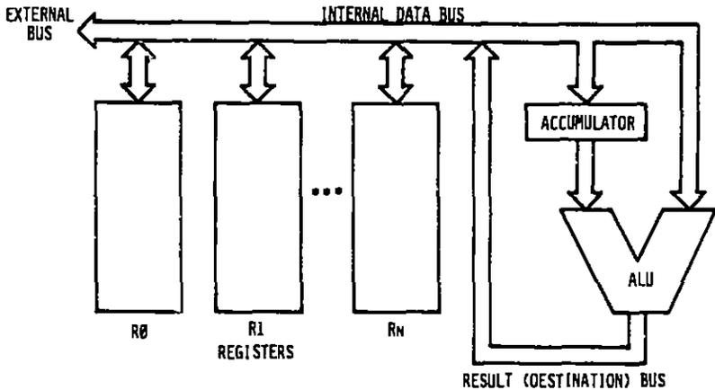
**Fig. 2.8: Single-Bus Architecture**
