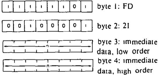
*Description:* The contents of the memory locations immediately following the opcode are loaded into the IY register. The low order byte occurs immediately after the opcode.
