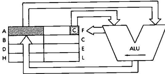
*Timing:*                      1 M cycle; 4 T states; 2 usec @ 2 MHz
