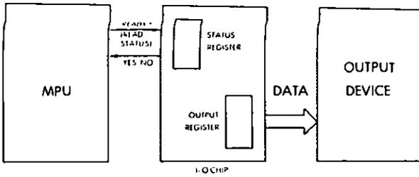
**Fig. 6.8: Handshaking (Output)**
