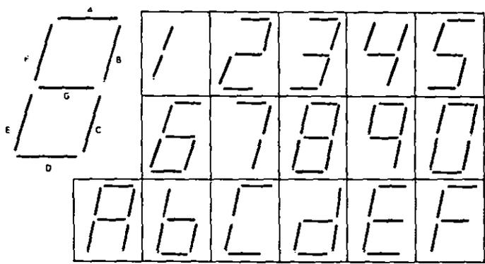
Fig. 6.11: Hexadecimal Characters Generated with a Seven-Segment LED
